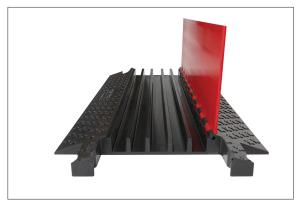
Protects cables/hoses up to 1.3" outside diameter, with a center channel accommodating up to 1.6" outside diameter.
